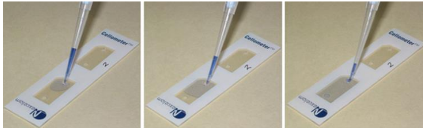
Capillary force automatically spreads cell sample within the counting chamber.
